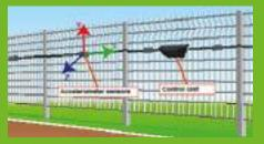
Accelerometer-based shock detection cable technology can detect movement in fencing or panelling in all three vectors (x, y, z). The acceleration of the three vectors combined, measures the desired signal intensity that will be used to trigger the alarm.
